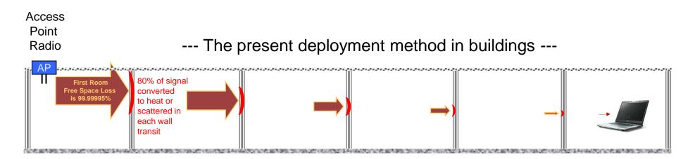
The signal level at the client notebook is only 0.000000005% of the original transmitted signal after going through a long span of free space and seven walls. Random and unreliable "hot spots" from reflections may allow temporary speed increases, but a slow and unreliable 1 Mbps data rate at the notebook's receiver is the most that can be expected. Low signals = low speed
