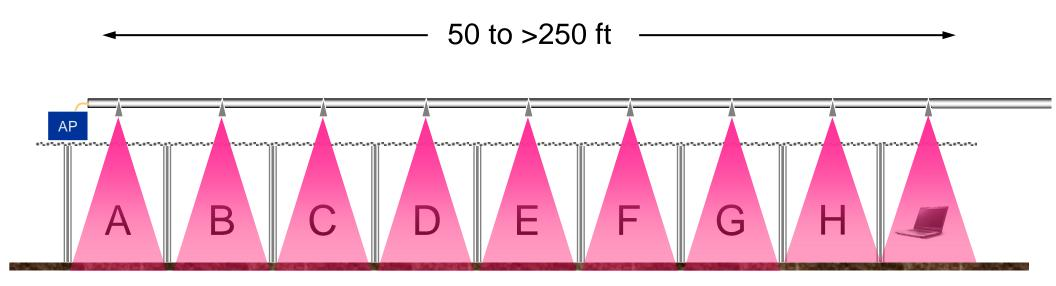
**RF** loss in the overhead distributing waveguide is <u>extremely low</u> with most AP signal power delivered to user areas, not wasted.
