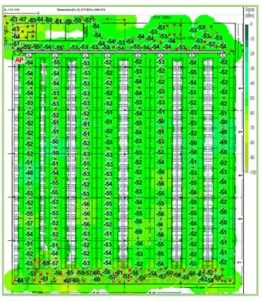
contents of shelves and provide reliable signals to personnel working in aisles and on docks.
